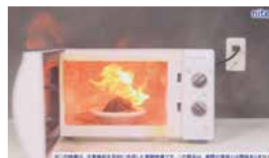
▲ A steamed bun ignited due to overheating by microwaving (Photo courtesy of National Institute of Technology and Evaluation)
