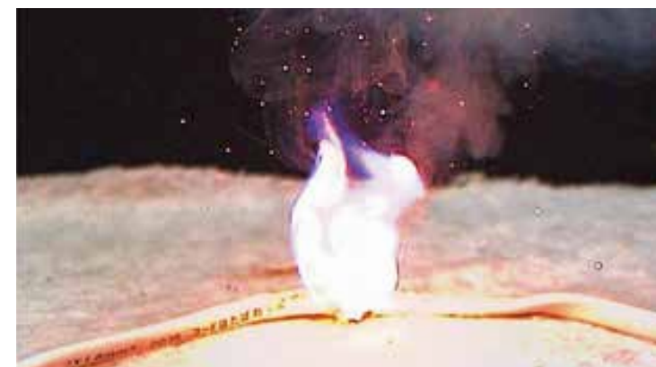
▲ A cut electric cord catches on fire (Photo courtesy of the National Institute of Technology and Evaluation)
