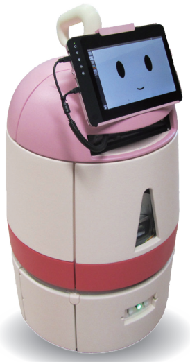
▲ Example of the application of a contact sensing cover (Patrol robot) (Photo courtesy of Mie Robot Exterior Technology Laboratory Co., Ltd.)
