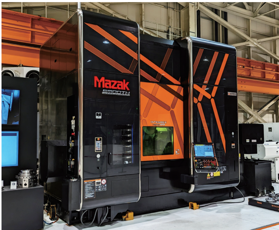
▲ An additive manufacturing machine, the winner of the Chubu Bureau of Economy, Trade and Industry Director General Award in the Monodzukuri Nippon Grand Awards / Development of hybrid compound processing machine equipped with grinding technology (Photo courtesy of Yamazaki Mazak Corporation)
