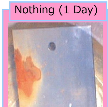
Workpiece's Rust (in Water)
