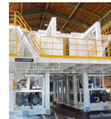
Back up trolley for shield machine with hydraulic unit
