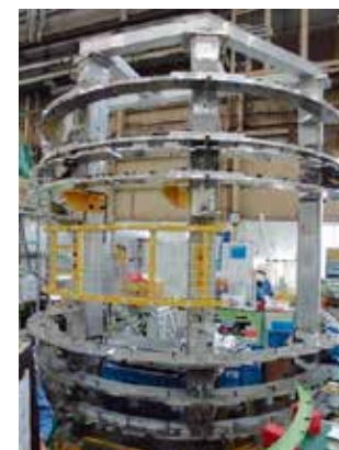
Jig for assembling framework of aircraft fuselage
