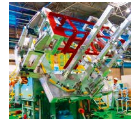
Jig for panel assembly of aircraft fuselage turning by hydraulic system
