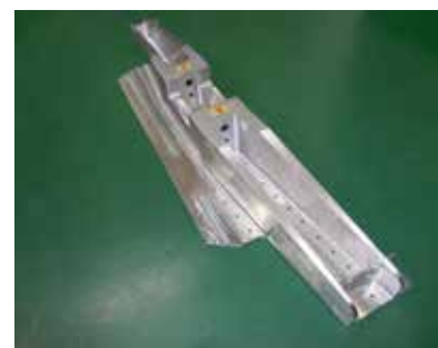
Aluminum part drilled with an angle head machine
